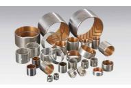
Bimetallic plain bearings withstand high load and shock conditions. For this purpose, a metallic overlay is sintered on a support plate. Depending on the application, different bronze alloys are available. These bearings are not maintenance-free and require good lubrication.
