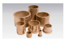
Sintered bearings are self-lubricating (oil impregnated), maintenance-free sintered products which can be produced in large quantities in accordance with DIN 1850-3 or ISO 2795 standard. They possess excellent storage properties due to the precision manufacturing and porosity of the sintered material in accordance with DIN 30910-3 standard. These bearings are intended for medium loads and higher sliding speeds.
