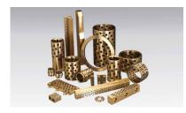
The plain bearings and sliding elements are made of casted bronze material in which a special solid lubricant is embedded. The base metal allows for high loads and the solid lubricant makes it possible to use the bearings without additional lubrication. Additionally, MBW-bearings perform exceptionally without lubrication, under conditions of low speeds and high load.
