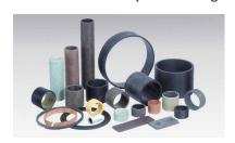
The reinforced composite structure enables the bearing to support high static and dynamic loads. They have an excellent shock and edge loading capacity, excellent corrosion resistance, and are dimensionally stable. These fibres reinforced composite bearings are available as bushes, plates, bearing segments and special forms depending on the particular material type.
