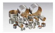
Bimetallic plain bearings withstand high load and shock conditions. For this purpose, a metallic overlay is sintered on a support plate. Depending on the application, different bronze alloys are available. These bearings are not maintenance-free and require good lubrication.
