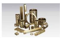
The plain bearings and sliding elements are made of casted bronze material in which a special solid lubricant is embedded. The base metal allows for high loads and the solid lubricant makes it possible to use the bearings without additional lubrication. Additionally, MBW-bearings perform exceptionally without lubrication, under conditions of low speeds and high load.
