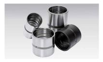
Hardened steel bushings are used for specifically high loads at low speed, e.g. in construction, agricultural and earth conveyer machines, demolition tools,
